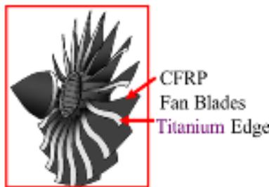
**Fig. 1:** Application of carbon fiber reinforced polymer (CFRP) with Ti sheath recently utilized for fan blades of turbo fan engines of airplane.
