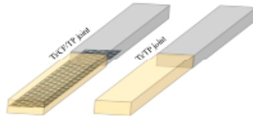
**Fig. 2:** Schematic diagram of joining samples with and without carbon fiber.
